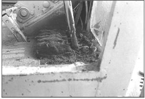
Prevent dirt from accumulating around the control valves. Valves in the condition shown above cannot operate properly. A clean machine reflects operator pride!
