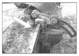
Accumulated debris will cause excessive wear on the shims. Keep the blade slide area clean.
