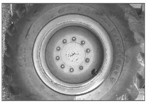
Check all lug nuts. Because of the vibration experienced during grading operations, lug nuts can become loose.
