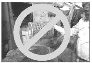
Do **NOT** bang the air filter against a tire or other object. Doing so will distort the shape of the filter, degrading the seal to the intake. If the filter is dirty, replace it!
