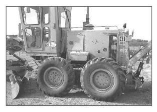
Mismatched tires cause internal wear on the drive chains and differential. Using mismatched tires does **not** save money.
