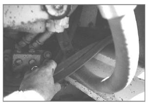
Check for hoses that touch other hoses. Hose contact causes abrasion that will eventually lead to failure.
