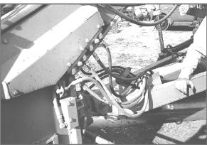
Hoses that have been replaced must be the proper length and secured in the same way as the originals.
