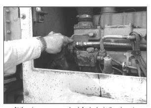
At the air compressor, check for leaks in the air system. Examine the compressor unit and all fittings and air lines. An accumulation of moist dirt is an indication of a leak.
