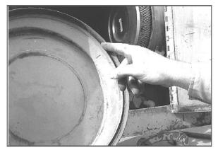
When servicing the air filter, check the gasket and the inner filter. If the gasket is damaged, unfiltered air can make its way through the system and into the engine.
