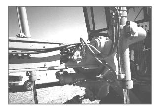
Loose hoses are a breakdown waiting to happen. Hydraulic hoses that have been added to the machine must be of the proper pressure rating and secured to the frame with clamps or brackets.
