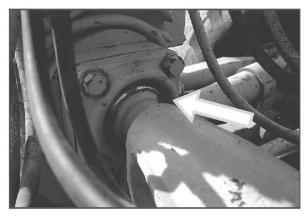
Check clearance of the drawbar ball and socket. Look for excessive free-play. Adjust if necessary.
