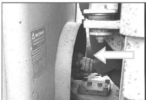
Be sure to replace the safety guard if you remove it to grease the drive shaft. The guard is there to protect you and your co-workers from injury.
