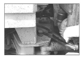
Keep the articulation area free of dirt, ice, and snow. Accumulated debris can knock off the water pump elbow, or damage the hood, cowling, or hoses when the machine is articulated.
