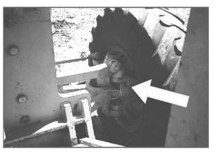
Check the spindles for excessive wear and play.
