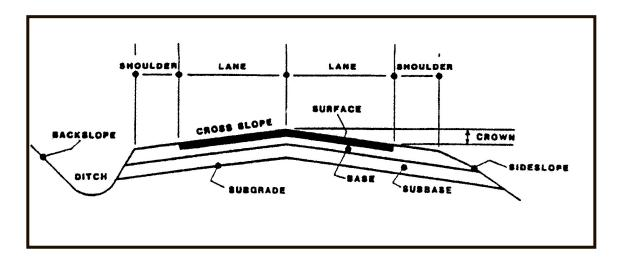
**Without** proper drainage, no roadway can survive. **With** proper drainage, you can maintain a stable base and keep a proper cross-section. And with a proper cross-section, the roadway, shoulder, inslope, ditch, and backslope will drain properly and your roads will be in better condition and easier to maintain under all weather conditions. Practice good maintenance habits and your time will be well spent.
