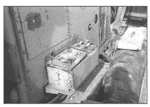
Keep the top of the batteries clean. Accumulated dirt attracts moisture, and this mixture can drain the battery's charge.
