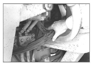
Hoses should be checked daily. Hydraulic hose failure is a major cause of motor grader breakdown.
