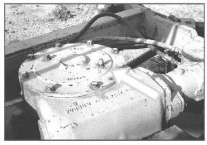
Keep the cover of the circle turn gear clean. This will allow the breather to function properly.
