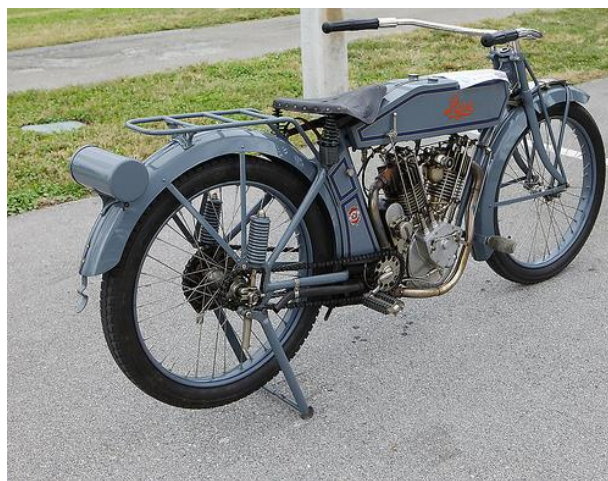
Figure 9 1913 Pope motorcycle with plunger system setup on the rear axle (Red)
