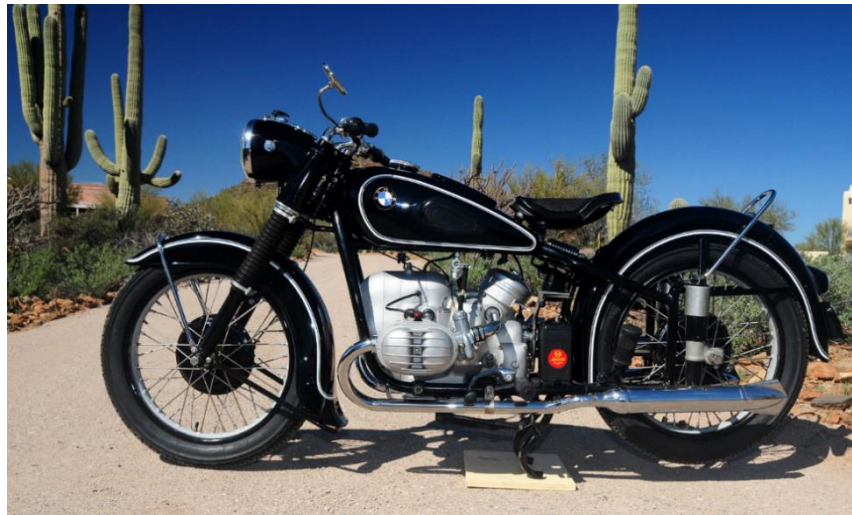
Figure 10 1951 BMW, note the plunger system at the rear axle (Dean)
