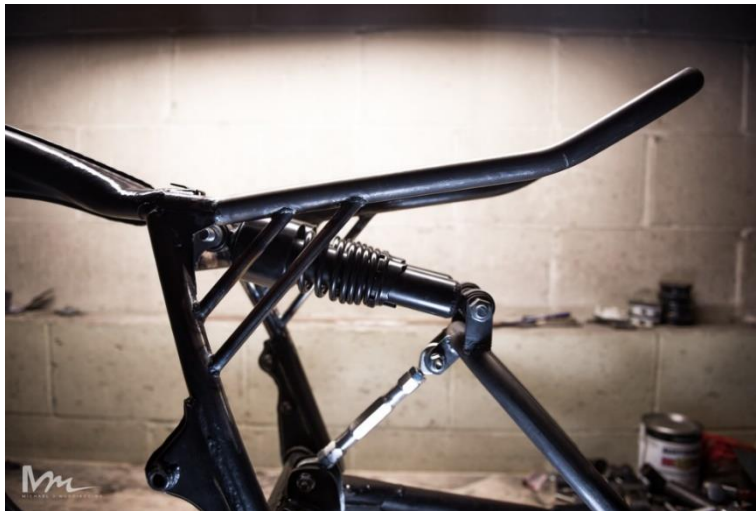
Figure 26 Kinetic Motorcycle suspension kit installed on frame with two shocks
