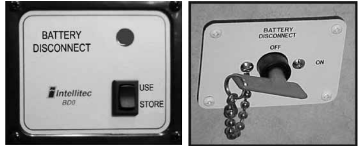
Battery Disconnect Switches
