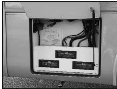
Rear diesel exterior electrical compartment fuse panel
