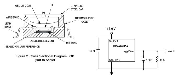
Figure 3. Typical Application Circuit (Output Source Current Operation)
