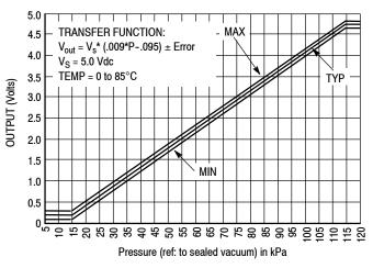
Figure 4. Output versus Absolute Pressure
