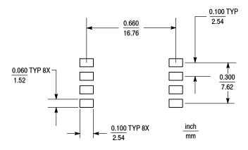
Figure 5. SOP Footprint (Case 482 and 482A)
