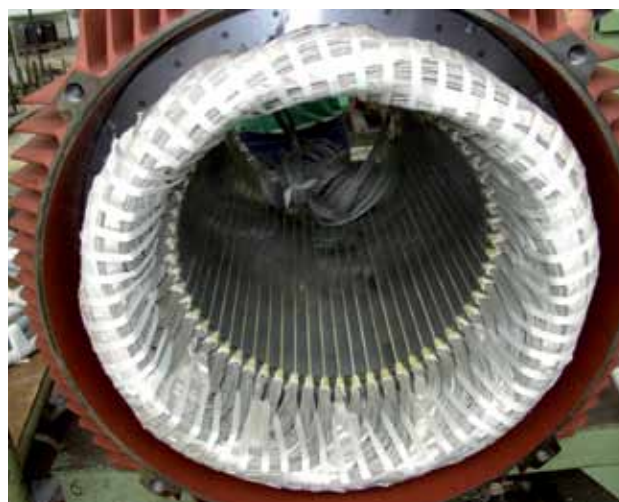
Fig. 4: Stator of the KV.R series, before impregnation
