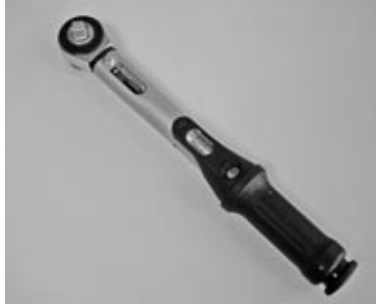
Torque wrench, measurement range 5 - 50 Nm
