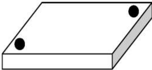
Diagonal gate: radial flow – twisting
