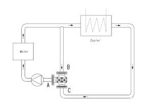
for the regulation of the medium-outlet temperatures as mixing valve, e.g.
