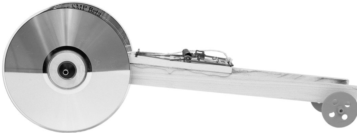
Figure 1: This sample mousetrap-powered vehicle has a large drive wheel and a small axle. The vehicle will move slowly and travel a long distance for each turn of the wheel.
