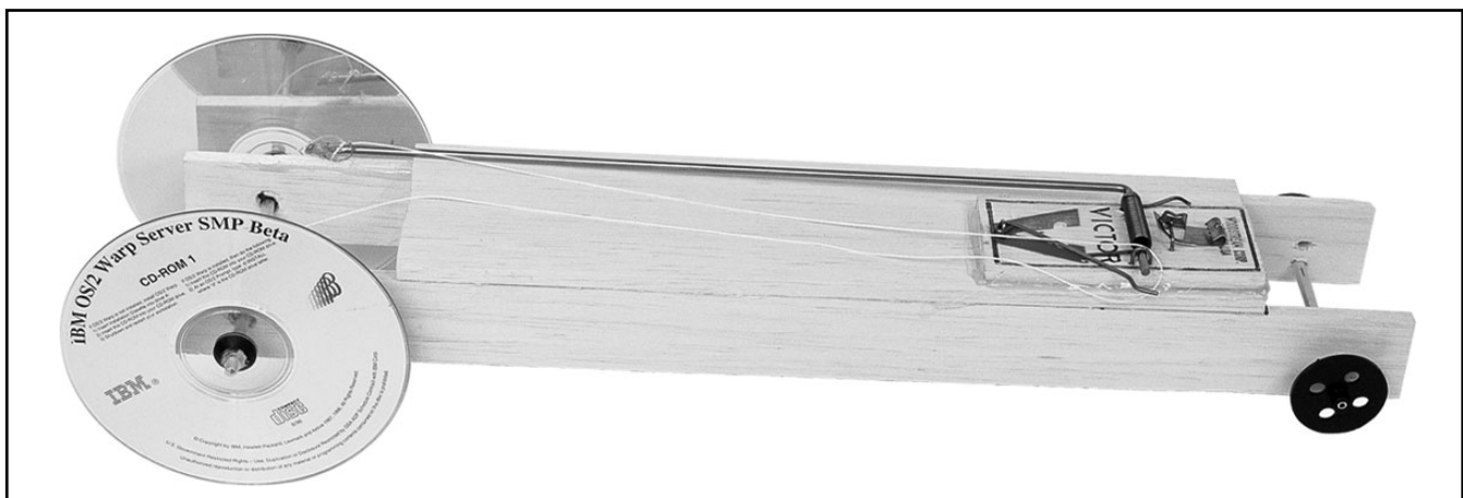
Figure 45: Basic vehicle with a long lever arm
