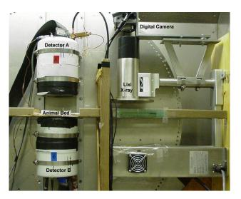
**Figure 3:** picture of the support gantry with two 110 mm PSPMT's and Lixi X-ray system.
