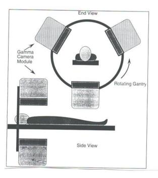
Figure 7: Diagram showing the operation of a clinical SPECT scanner
