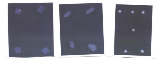
**Figure 12:** Example of different reflectors. The far left image shows 3M Scotchlite reflectors. The middle image shows glass bead reflectors. The right image shows White Out as a reflector.
