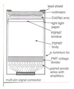
Figure 1: Position Sensitive Photomultiplier Tube
