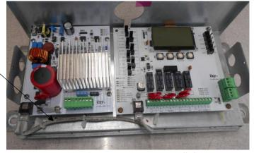
Figure 15 -ECI MOVFR LCD Installed
