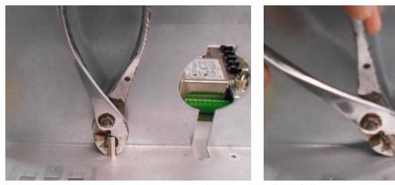
Figure 12 - Snapping Off Standoff
