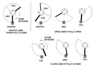
Figure 24 - Left Hand CAM Settings
