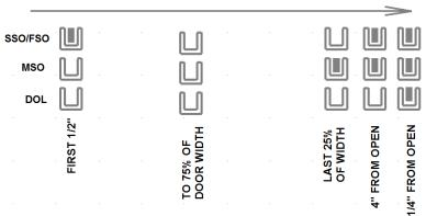
Figure 22 - OPEN CAM/SENSOR Sequence
