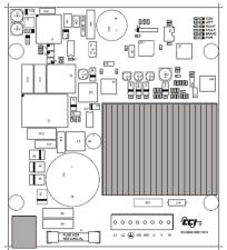
Figure 8 - Variable Frequency Drive Board
