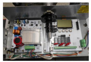
Figure 18 - ECI MOVFR-LCD Installed
