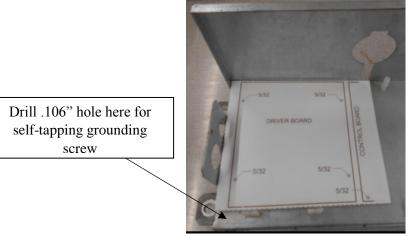
Figure 13 - Drill Pattern placement
