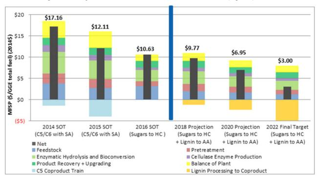
Figure 1. Cost projections for low-temperature deconstruction and catalytic upgrading of sugars pathway. To reach an MFSP of \$3/GGE, the lignin waste stream must be converted into a value-added product (in this case, adipic acid)<sup>1</sup>.
