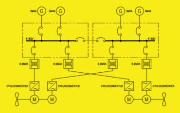
FIGURE 1: Existing propulsion one-line for a Jumbo Mark II.
