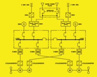
FIGURE 3: New hybrid one-line for a Jumbo Mark II.
