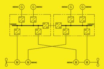
FIGURE 2: Typical hybrid DC propulsion one-line.
