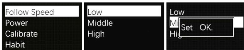
5. Power: Motor torque adjustment, please keep the original parameters.
