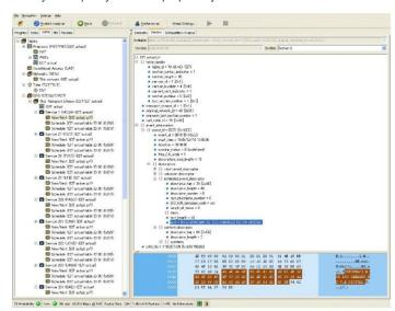
Tables and their data source are displayed. This shows the data bytes (in both hexadecimal number format and ASCII character format), for the selected table, version, and section. Tables and subtables are easily analyzed and directly traceable to packet data.
