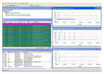
There are two types of buffer model; the one to use by the receiver is signaled within the Elementary Stream itself. The T-STD method is based upon the DTS values within the PES header and can be used for any contained CODEC type. Additionally, certain video CODECs such as MPEG-2, MPEG-4 (AVC) or HEVC (H.265) may contain buffer parameters within the ES itself.
