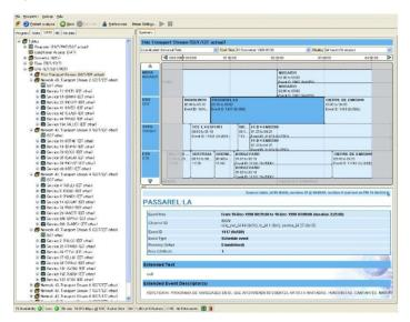
**Event panel** – The event panel shows the events for one or more services, depending on the node selected. Individual events are color coded and shown as blocks. Each block (and its associated tooltip) displays event information extracted from the EIT. When a block is selected, the complete event information is shown in the Event detail panel, including a link to the section carrying the information. Events are color coded as follows:
