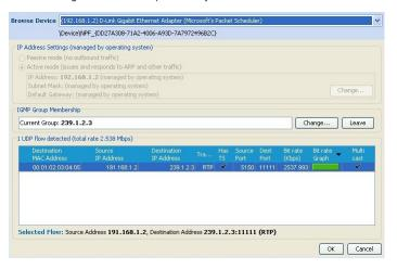
UDP sessions carrying MPEG TS traffic are indicated and may be selected for analysis and recording. Transport Stream packets are time stamped as they are received from any Network Interface Card, allowing PCR measurements and graphing to be supported. In addition, a display of the mean IP Packet Interarrival Time (PIT) histogram is available.
