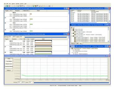
Use the Multiplexer/Remultiplexer/Demultiplexer application to create multiprogram Transport Streams with custom SI/PSI/PSIP information for DVB (including Annex A string support), ATSC, ISDB, and MPEG compliant Transport Streams including ISDB-T Single Segment mode.
