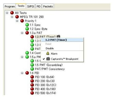
The captured stream can also be permanently stored on the hard disk for subsequent reanalysis with the deferred time TSCA application. This powerful debug mode enables fast debugging of troublesome intermittent problems. CaptureVu technology also supports triggering events based upon IP Layer measurements, providing integrated cross-layer fault analysis and logging in a single box solution for network fault diagnosis.
