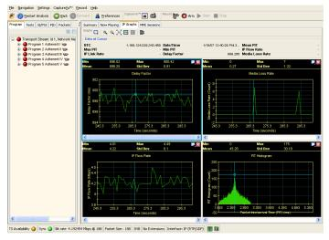
PCR graphs are available in real time and deferred time. Time stamping data makes sure that these can be captured and viewed on stream recordings. Selectable MGF filters provide maximum flexibility and compatibility in these important PCR measurements. The TSCA is also able to display PTS Arrival Interval graphing in real time or deferred time and includes PTS-PCR and DTS-PCR graphs to detect possible Receiver buffer under- and overflow problems.
