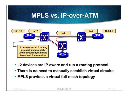
This figure illustrates how MPLS is used in ATM networks to provide optimal routing across L2 ATM switches. In order for MPLS to work with ATM switches, the switches must be somewhat L3 aware. The ATM switches must run a L3 routing protocol and thus have knowledge about how to reach L3 subnets.
