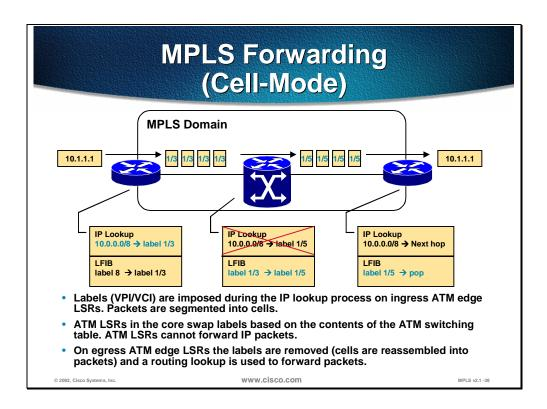
Cell-mode MPLS is similar to frame-mode MPLS. The difference is that ATM LSRs (ATM switches) are not capable of forwarding IP packets:
