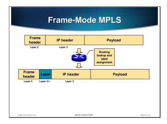
This figure illustrates an edge router that receives a normal IP packet. The router then performs the following actions:
