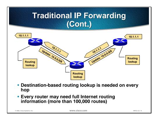
This figure illustrates how routers in a service provider network forward packets based on their destination addresses. The figure also shows that all the routers need to run a routing protocol (BGP) to get all the Internet routing information.
