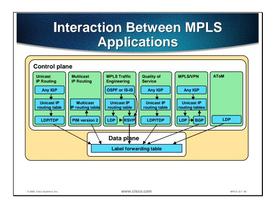
This figure illustrates the complete architecture when all applications are used. Each application may use a different routing protocol and a different label exchange protocol, but all applications use one single label-forwarding engine.
