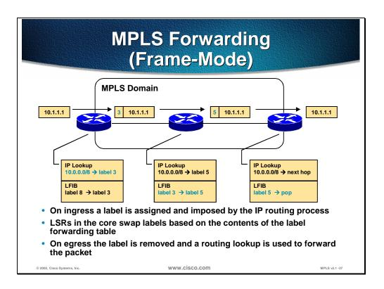
This figure illustrates an MPLS network using frame-mode MPLS. All LSRs are capable of forwarding IP packets or labeled packets. The ingress edge LSR performs a routing lookup and assigns a label. The middle router simply swaps the label. The egress LSR removes the label (penultimate hop popping is covered later) and optionally performs a routing lookup.
