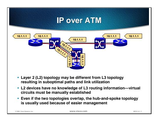
This figure illustrates a worst-case scenario where Layer 2 (L2) and Layer 3 (L3) topologies do not overlap. The result is that a single packet could be propagated with three L2 hops but instead requires 7 hops. The reason is that L2 devices have static information about how to interconnect L3 devices. Routers use a routing protocol to propagate L3 routing information through the intermediary router.
