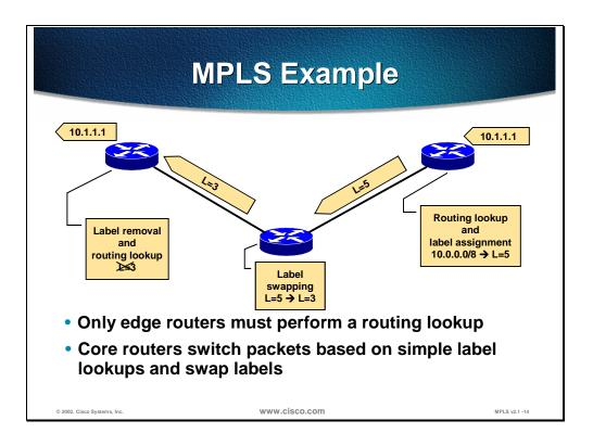
This figure illustrates a situation where the intermediary router does not have to perform a time-consuming routing lookup. Instead this router simply swaps a label with another label (5 is replaced by 3) and forwards the packet based on the received label (3).
