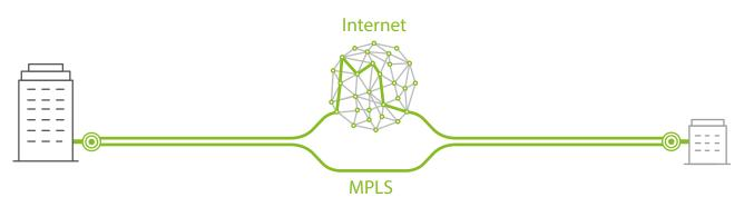
SD-WAN solutions offer the management capabilities to direct the relevant traffic according to its required class of service, offloading MPLS links and delaying the need to upgrade capacity. SD-WAN solutions, however, are limited in a few key aspects:
