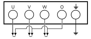
Figure 22. Hard Wire Hookup for Single Phase 277V, 254V, or 240V
