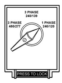
Figure 27. Voltage Selector Switch 240/120V Single Phase Position
