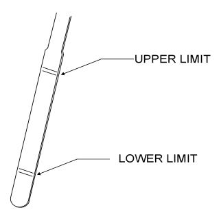
Figure 31. Engine Oil Dipstick
