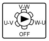
Figure 12. AC Voltmeter Change-over switch (Reading the W-U leg on the output terminal panel)
