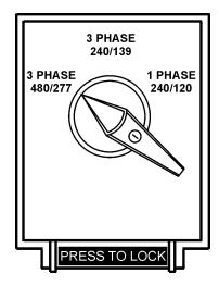
FIGURE 17. Voltage Selector Switch 480/277V Three Phase Position
