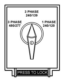
FIGURE 23. Voltage Selector Switch 240/139V Three Phase Position
