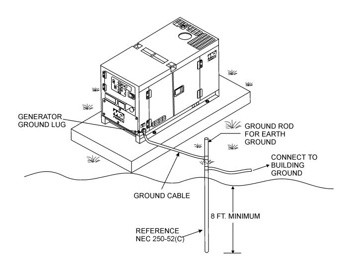
Figure 30. Typical Generator Grounding Application
