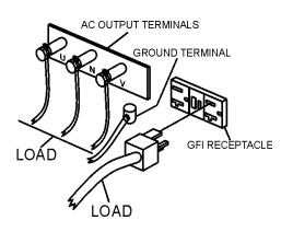
Figure 35. UNV Terminal Lugs (Load)
