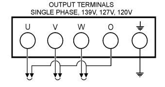
Figure 26. Hard Wire Hookup for Single Phase 139V, 127V, or 120V
