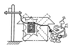
■ Backfeed to a utility system can cause electrocution and/or property damage. Do not connect to any building's electrical system except through an approved device or after building main switch is opened.
