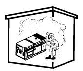
The engine of this generator requires an adequate free flow of cooling air. Never operate the generator in any enclosed or narrow area where free flow of the air is restricted. If the air flow is restricted it will cause serious damage to the generator or engine and may cause injury to people. The
