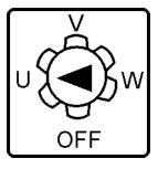
Figure 14. AC Ammeter Change-over Switch (Reading the U leg on the output terminal panel)
