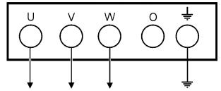
Figure 20. Hard Wire Hookup for Three Phase 480V, 440V, or 416V
