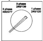
Figure 38. Voltage Selection Switch
