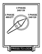
Figure 11. Voltage Selector Switch 240/120V Single Phase Position
