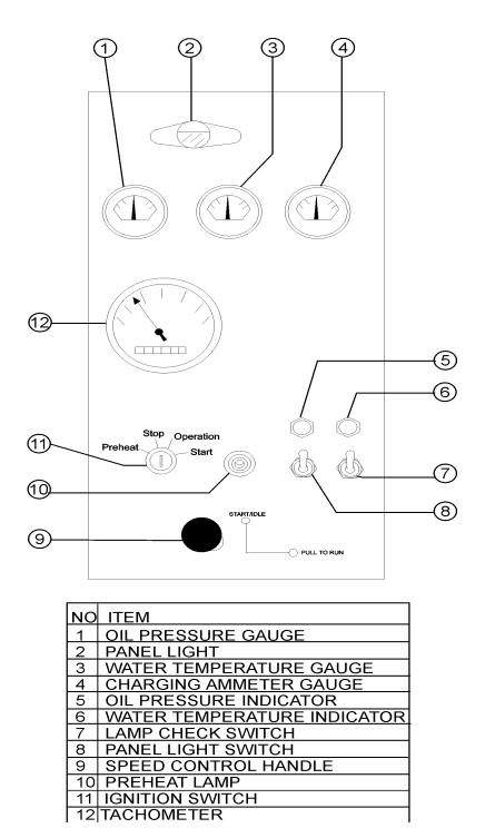
**Figure 7. Engine Operating Panel**
