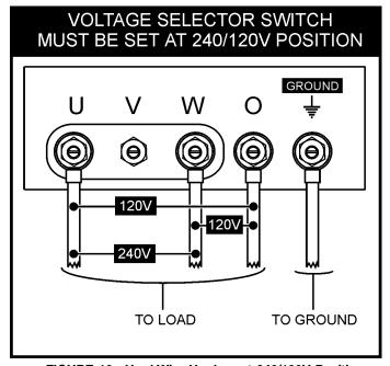
FIGURE 16. Hard Wire Hookup at 240/120V Position
