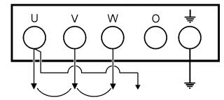
Figure 21. Hard Wire Hookup for Single Phase 480V, 440V, or 416V
