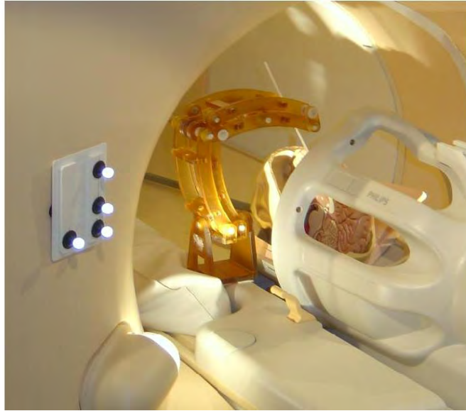
Figure 1.1: The prototype robot in the bore of a 3T MRI scanner with the cannula targeting a model skull
