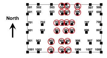
Figure 8. Core columns estimated to be heavily damaged or destroyed in numerical simulation.
