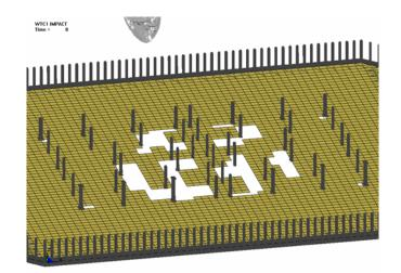
**Figure 7.** Story 95 cut-out showing the core columns, floor slab, and perimeter columns along the south and north faces of WTC-I. Incoming aircraft can be seen on the north side.
