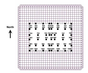
Figure 6. Floor plan of WTC-I showing 47 interior (core) columns and 240 exterior
