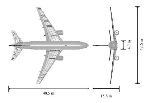
Figure 1. Overall dimensions of Boeing 767-200ER.
