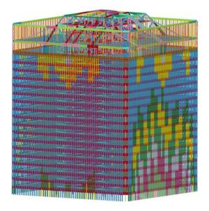
Figure 3. Elevation of the WTC-I model.
