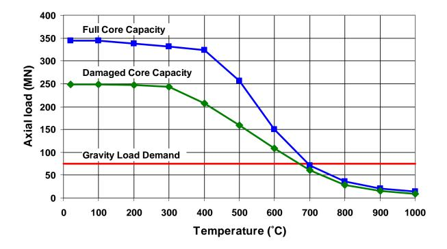
**Figure 11.** Axial load capacity of core columns and estimated gravity load demand at story 95 of WTC-I.
