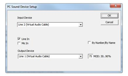
Audio Setup for Apache Labs Anan 100D: Use 0 dB Gain on VAC TX / RX, adjust using Windows Sound Mixer for 50% output (50w)
