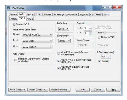
Balance the MS-DMT (MIL-STD Data Modem Table) and FLDIGI output levels so the same VAC gain can be used (0 dB).
