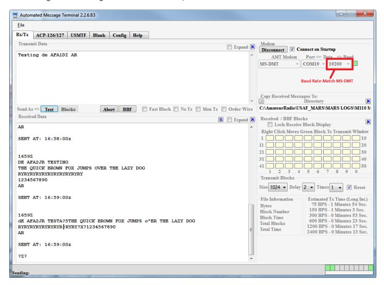
The DATA PORT used is COM19 at 19200 baud, same baud rate as the DATA PORT COM9 for MS-DMT.
