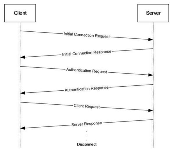
Figure 13: Client connection use case
