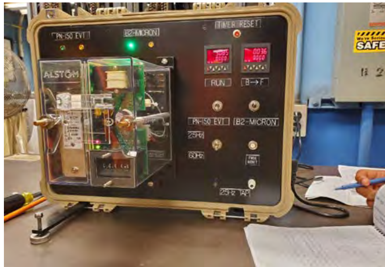
Figure L-1. NYCT TCTUR with Alstom B2 Micron Relay.
