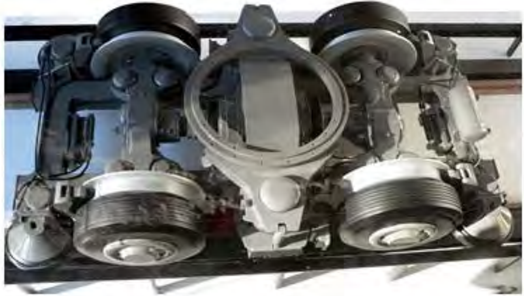
Figure 12: Paris Metro Truck, with Rubber Tires Installed
