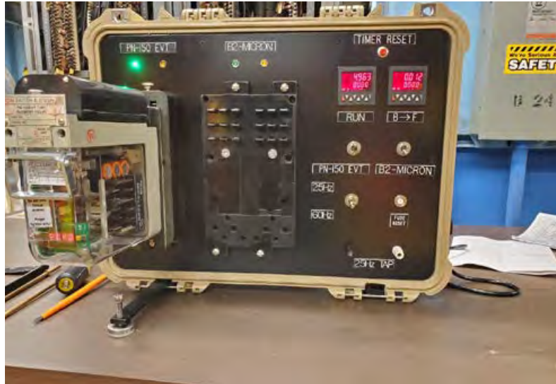
Figure L-2. NYCTY TCTUR with Ansaldo PN-150 EVT Relay.
