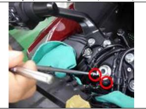
11. Remove the left rear handlebar bolt and washer [1].
