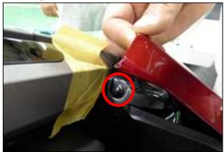
6. Lift the ends of the top shelter just enough to remove the socket bolts from the center panel switch (left and right sides, two bolts total).
