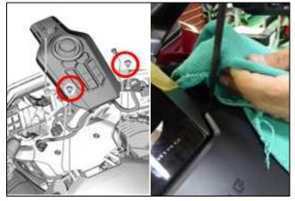
7. Wrap the rear part of the center panel switch with a clean cloth.
