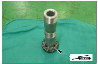
3. Install the dust seal [1], lower inner race [2], and lower steering bearing [3] onto the stem shaft [4].
