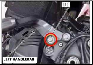
12. Loosen the handlebar bolt [1], move the handlebar forward enough to make the tie rod nuts accessible for a socket, then retighten the handlebar bolt to hold the handlebar in its new temporary position.
