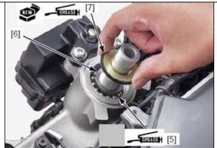
5. Apply the specified grease to the threads of the adjustment nut. Hold the stem and tighten the adjustment nut [1] to the torque specified below.
