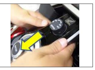
13. Lift the end of the top shelter and install the socket bolts for the center panel switch (left and right sides, two total).
