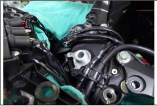
3. Apply the specified grease to the steering stem nut threads [1]. Install the steering bridge [2], washer [3] then install and tighten the stem nut [4] to the specified torque below while holding the stem shaft.
