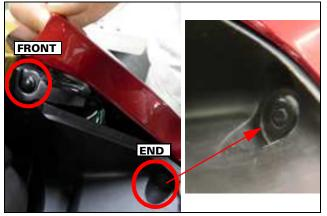
15. Push the end of the top shelter down until it snaps into place. Verify the front tabs are engaged in the slots of the speaker grill before pressing the top shelter in place.
