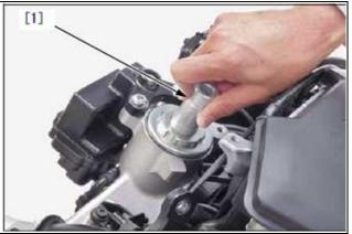
7. Recheck the adjuster nut [1] tightness to the specified torque below then recheck that the steering stem moves smoothly without play or binding.
