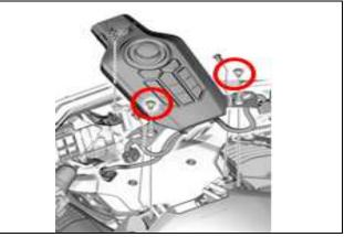
14. Lift the end of the top shelter. First, install a trim clip at the front of the center panel switch (left and right sides, two total). Next, install a trim clip in the end of each top shelter (left and right sides, two total).
