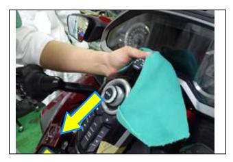
12. With the center panel switch moved forward, insert the clip at the front part of the center panel switch. Slide the center panel switch toward the rear of the motorcycle.
