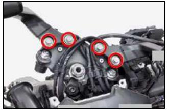
9. Install the cable clamps and cable clamp bolts then tighten each bolt to the specified torque below (left and right sides, two total).
