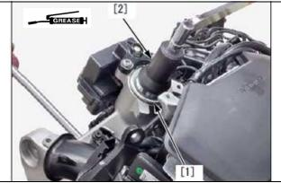
6. Rotate the stem shaft [1] five times to seat the bearings.
