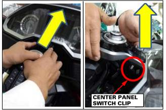
Remove the screws [1] from the top bridge cover [2]. Disengage the cover by lifting the rear of it then disengaging the front. Rotate center panel switch backwards, resting it on a clean towel. Note how cables and hoses are routed in the cover for re-assembly.
