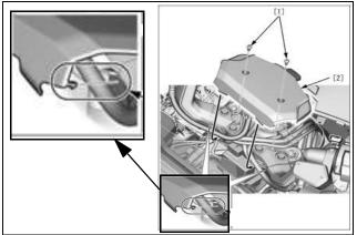
11. Lift the left and right ends of the top shelter to protect the center panel switch as you slide it into position.
