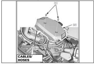
10. Remove the cable clamp bolts and cable clamps (left and right sides, two total).
