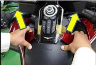
4. Protect exterior parts by covering the speedometer and top shelter with clean shop towels in the areas shown below.
