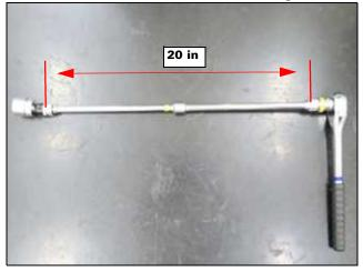
17. Using the assembled tool (previous step), hold the stem shaft from underneath.
