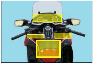
5. Lift the end of the top shelter, then remove the trim clip on both sides of the center panel switch (left and right sides, two clips total).
