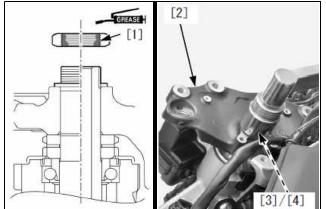
4. Wipe off any extra grease thoroughly after tightening the stem nut. Make sure the stem shaft moves smoothly without play or binding.
