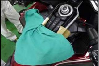
8. Push the center panel switch forward, towards the meter panel, then lift the front of it up to disengage from the front mount. Disengage the clip at the front of the center panel switch (shown below).
