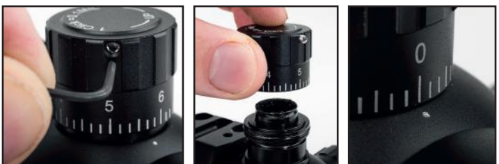
Figures 3a/3b/3c: Loosen the turret grub screws to freely rotate the vernier to the “0” position
