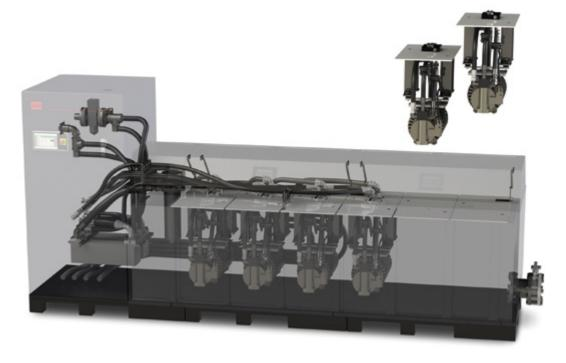
The new SilentFlo 515 HPUs are quiet and easy to operate. The covers are lower than previous generations to enable easier access. The new molding technology used to make the covers results in better sound absorption and quieter operation, and the gas struts make it simple to raise the cover.
