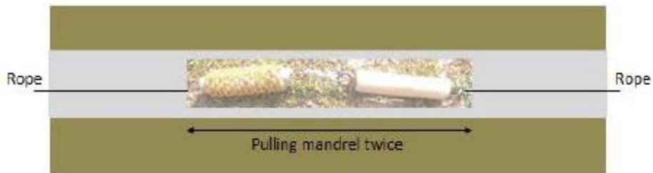
Figure 24. Pulling mandrel from both directions
