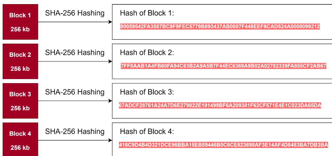
Figure 17: An example of hashing data blocks by the SHA-256 algorithm
