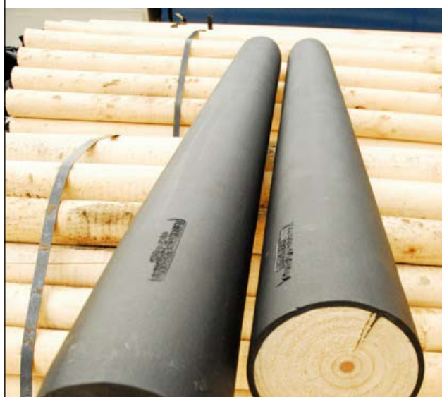
FIGURE 8.8 Wooden posts with synthetic cover to prevent marine organisms boring into them
