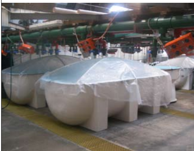
FIGURE 4.8 Larval rearing tanks covered with plastic to control aerosol contamination and assist in temperature control
