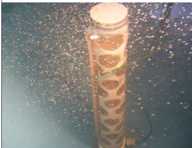
FIGURE 4.11 Aeration device around central standpipe in mud crab larval rearing tank designed to keep larvae in suspension within the water column
