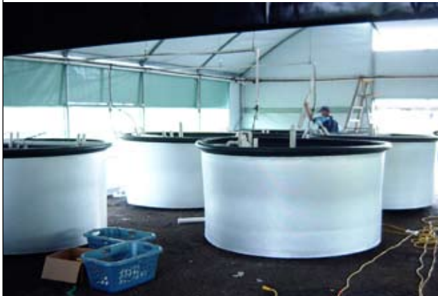
FIGURE 4.7 A mud crab hatchery with ventilation provided by windows, doors and vents, with tanks that are wrapped in insulation to assist in temperature control
