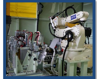
Exhaust System Welding Line
