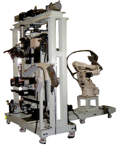
CO2 Welding for Main Exhaust System
