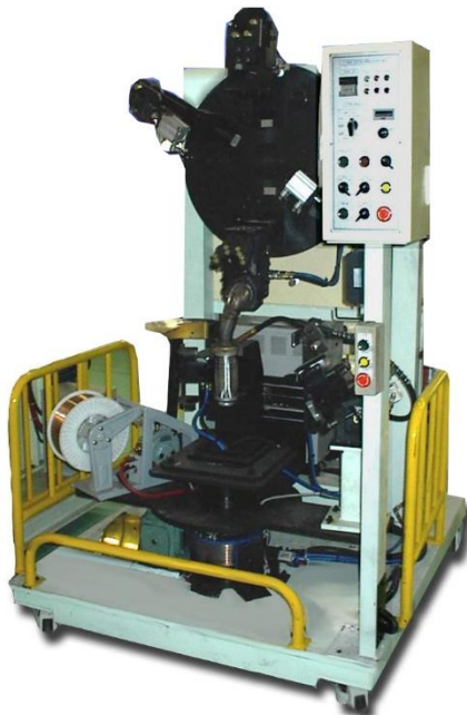
CO2 Welding for Exhaust Pipes and Flanges
