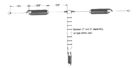
**Figure 1** - Schematic drawing of the W5GI Multi-band Mystery Antenna. See text for details on connection of coax sections in center of antenna legs and on length of of twin lead stub.
