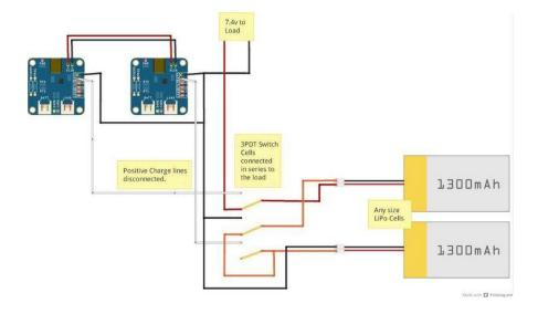
Since the cells are not guaranteed to be balanced during the fast-charge, it is best to wait until both cells are fully charged before switching to Run mode.
