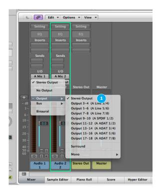
2 Set the software application's mixer output to Out 1-2 (Stereo Output).
