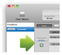
A device icon and ID button is placed adjacent to each row of parameters to identify the hardware unit to which the row belongs. By clicking on the ID button, the corresponding hardware unit's front panel will illuminate. Each hardware unit is assigned a Peripheral Prefix (A-Z, found in Maestro's Device Settings tab window) which is displayed on the ID button.
