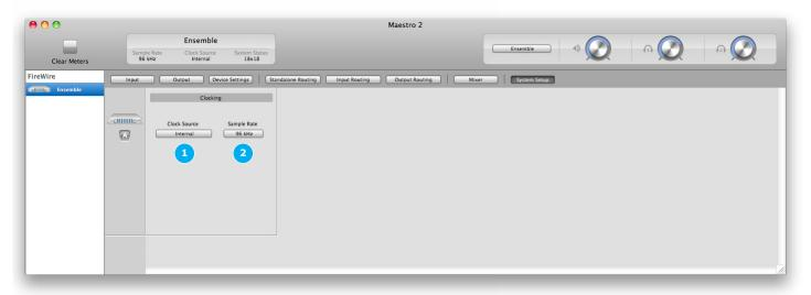
1 Clock Source - This drop down selects the clock source for the Ensemble.
