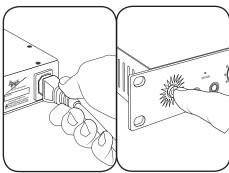
Connect Ensemble's AC input to an AC outlet of 90 to 250 volts; Ensemble's power switch will illuminate to indicate the presence of AC. Press the power switch to turn the unit on (figure 3).
