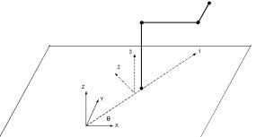
Figure 1 Structure subjected to two horizontal components applied along any arbitrary directions and the vertical component seismic motion
