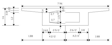
Figure 4 Typical section of superstructure
