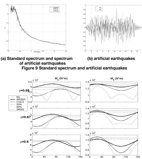
Figure 10 Reaction forces of pier 4 using various methods for standard spectrum (Time history analysis, CQC3 method, SRSS, percentage rules)
