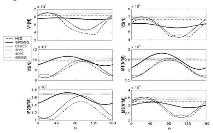
Figure 8 Reaction forces of pier 4 using various methods (Time history analysis, CQC3 method, SRSS, percentage rules)
