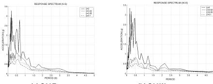
(a) S00E component (b) S90W component Figure 7 Acceleration response spectra for EL CENRO earthquake
