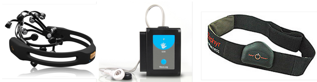
Figure 1. The EEG, GSR, and HRV sensors used in the experimental setup.
