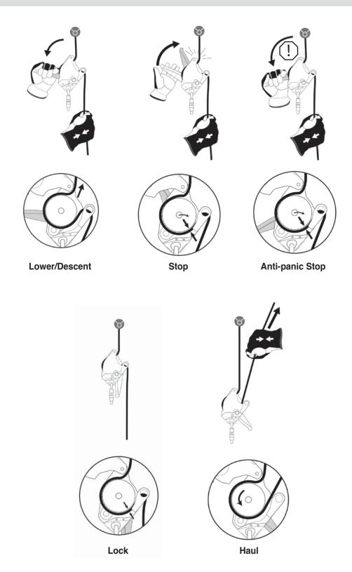
The CLUTCH allows the rope to be pulled through in one direction, but friction of the rope on the Sheave in the other direction causes the Sheave to lock, pivot and capture the rope between the Sheave and Friction Shoe. By holding the braking side of the rope, the Brake Hand helps engage the braking mechanism.
