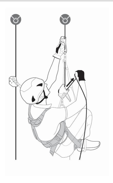
Attach the CLUTCH to the harness with the Control Handle in the Stand By position. For greater efficiency, take up slack as you stand up using the Rope Grab. Never allow slack between the Rope Grab and the CLUTCH.
