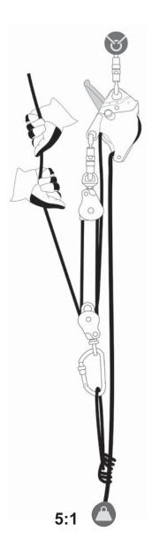
Add an appropriate rope grab and traveling pulley to the working rope, and if desired a second change of direction pulley to the Becket of the CLUTCH, to build simple or compound mechanical advantage systems.
