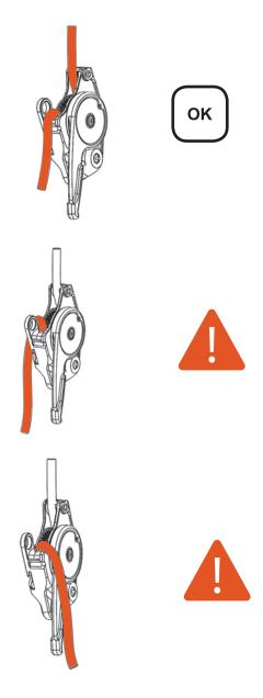
**WARNING:** When lowering, the tail of the rope should pass over the Friction Shoe, located adjacent to the Becket. Avoid placing the tail over the Sideplate or over the back of the Chassis.
