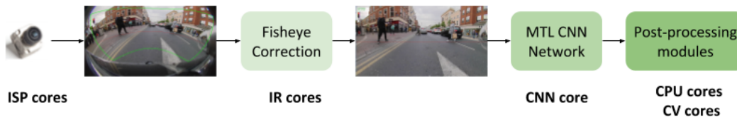
Figure 1: Video pipeline on the SoC
