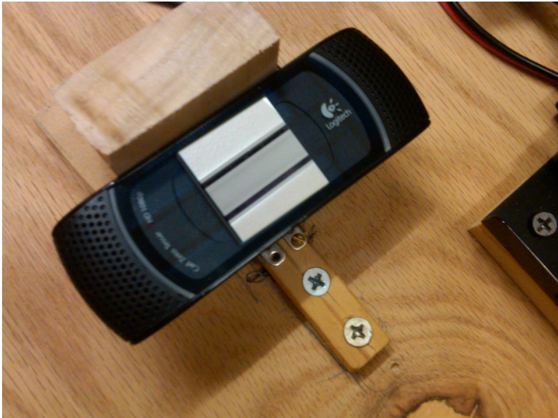
Figure 52 - Placement of IR Filters over camera
