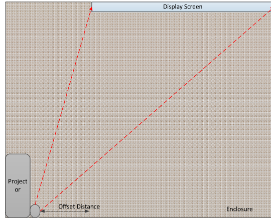
Figure 20 - Mounting option of Short Throw Projector with Offset greater than 100%
