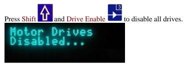
When the drives associated with servo systems are disabled, the power to the motors is also disabled. The motors associated with stepper systems still have power after the drives are disabled, but there is no output from the control board.
