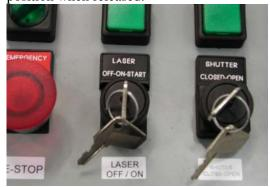
6. Rotate the Shutter key clockwise to open the shutter.
