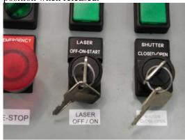
5. Rotate the Shutter key clockwise to open the shutter.
