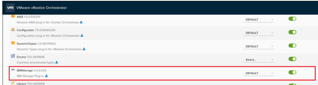
Figure 30 Successful installation of IBM Storage Plug-in in VMware vRealize Orchestrator
