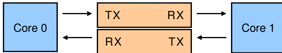
Figure 3.6.1.2: Two data buffers used for signal exchange.
