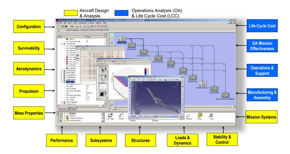
MDAO framework systematically links CAD and analytical systems, with Life Cycle Cost and Operations Analysis, to provide a more disciplined approach
