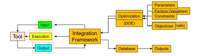
Once the design space has been explored, a variety of Optimization techniques may be applied to find local/global maximums and minimums of some specified objective function, subject to given constraints, in the design space
