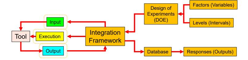
Once the design process is automated, this enables Design Space Exploration with a variety of Design of Experiments (DOE) techniques
