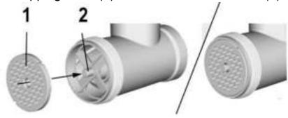
Notes: match the notch on the grid with the lug on the chopper. It is possible to choose; Fine, medium or large grid.
