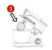
Install the accessory (whip or hook or beater) on the axis of the robot by engaging it.
