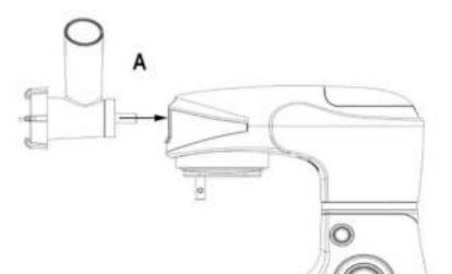
When the mincer is inserted in the appliance, the logo (triangle) located on the mincer must be opposite the logo (triangle + open padlock) of the appliance (1).
