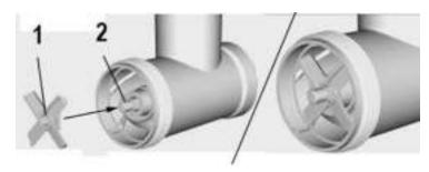
Install one of the chopping discs (1) in front of the knife blade (2).
