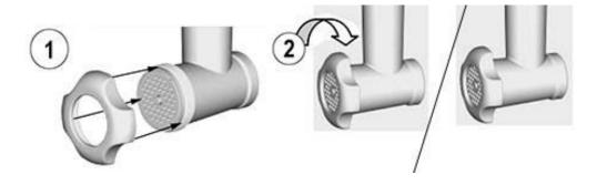
Insert the chopper on the front of the appliance. To do that : Tilt the chopper tube 25  $^{\circ}$  to the right and enter the chopper shaft into its place. (A)
