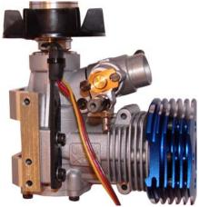
RPM sensor mounted on motor
