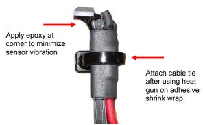
Completed RPM sensor mounted on bracket
