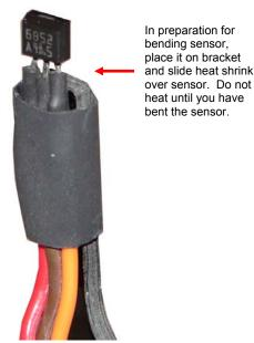
Heat shrink wrap on RPM sensor and bracket
