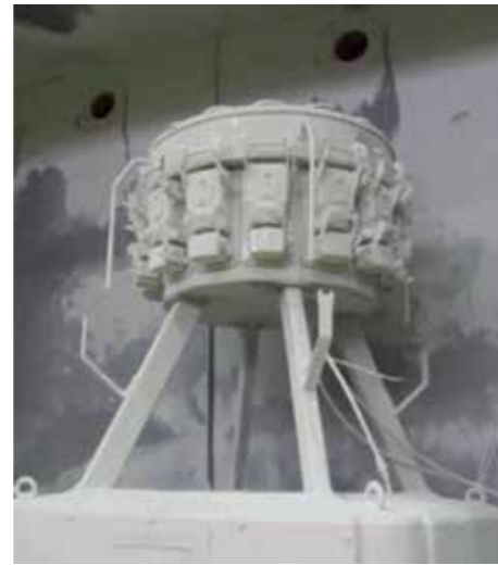
Dust test for IP6X
