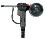
Spoolmate<sup>™</sup> 100 Spool Gun 300371 Direct-connect spool gun handles .030-.035 inch (0.8-0.9 mm) aluminum (4043 only) and .023-.035 inch (0.6-0.9 mm) steel/stainless steel wires. Rated at 135 amps, 30-percent duty cycle. Includes 12-foot (3.7 m) cable assembly and custom carrying case.
