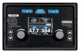
Auto-Set<sup>™</sup> Elite fast and easy predefined settings for multiple materials and processes to help you get welding quickly.
