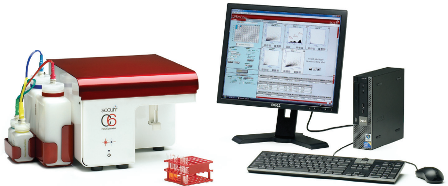
The BD Accuri C6 cytometer system.
