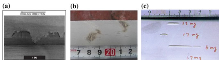
Fig. 1 Example defects on final steel products: a sliver [9], b scab [10], and c blister defects [9]
