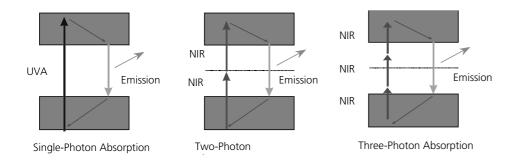
Fig. 8-1 The principle of multiphoton excitation
