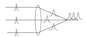
Fig. 8-12 Schematic pulse transformation by a singlet lens showing the influence of chromatic aberrations on the peak intensity due to Propagation Time Difference (PTD).
