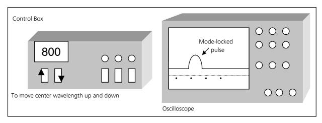
Fig. 8-6 Schematic of a IST Rees Spectrum Analyzer
