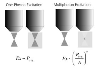
Fig. 8-2 One-photon vs. Multiphoton excitation. Two images of an objective are shown for each example. In each case, the first indicates the shape of the focused beam after passing through the objective. The second indicates the fluorescence that would be observed if the beam was focused through a cuvette containing a homogeneous solution of fluorescent dye.
