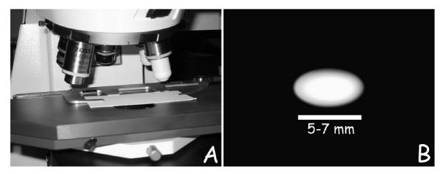
Fig. 8-10 (A) Setup for checking the beam alignment; (B) Optimal shape of the NIR laser spot
