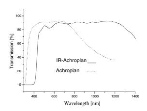
Fig. 8-13 Typical transmission curves of an IR-Achroplan and an Achroplan.
