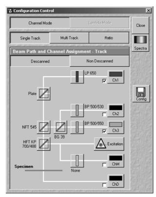
Fig. 8-11 Configuration for testing the overlay of the grid reflection images gained with the vis (543 nm) laser and the NIR laser
