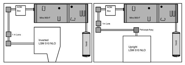
Fig. 8-4 Typical alignment scheme for the LSM 510 NLO direct-coupled system using and inverted (left) or upright (right) microscope.
