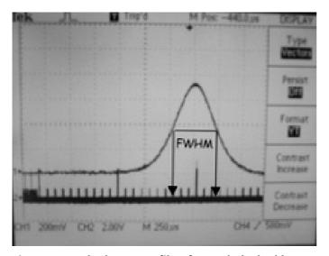
Fig. 8-9 The beam profile of a mode-locked laser output. The bandwidth of the pulse is the full width at half maximum (FWHM) of the bell shaped curve. In this case the bandwidth is approximately 6 nm, which is ideal for direct-coupled systems.
