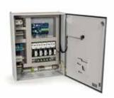
The ACS-30 PCMs provides power connection, with built-in electrical safety devices, line current sensing, alarming, switching (electromechanical relays) and RTD inputs for the heat-tracing circuits when used with the UIT. The ACS-30 PCM enclosure is rated IP54 to EN60439 and is approved for nonhazardous indoor or outdoor locations.
